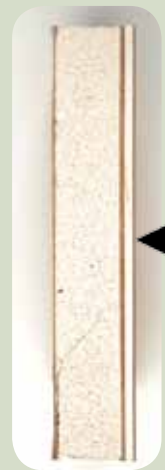
Induro™ FRP wall panel - nominal damage to subwall
