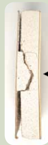
Rigid plastic wall panel - hidden failure of subwall
